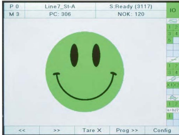
Figure: A full-screen smiley is an internationally understood symbol for the global OK/NOK evaluation (alternatively can display PASS/FAIL).
