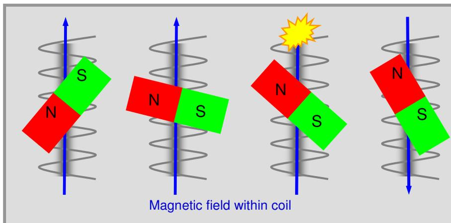
Figure 5: Wiegand effect: as the external magnetic field changes, a sudden change in the polarity of the ferromagnetic material is triggered
