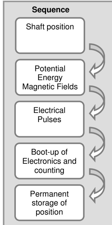
Figure 6: Turn-counting powered by the Wiegand effect.
