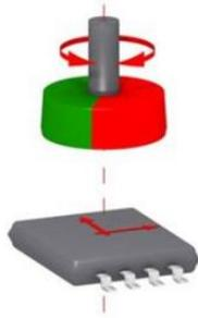
Figure 3: Hall effect sensor for an absolute magnetic encoder
