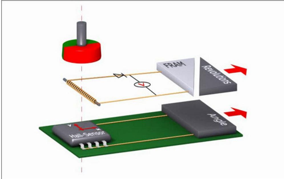
Figure 4: Hall sensor, plus Wiegand effect turn counter.
